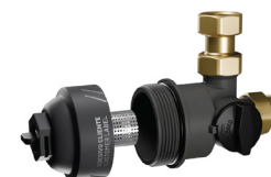
Fig. 7. ADS 100 dirt separator emptied of medium and with dirt collector unscrewed
