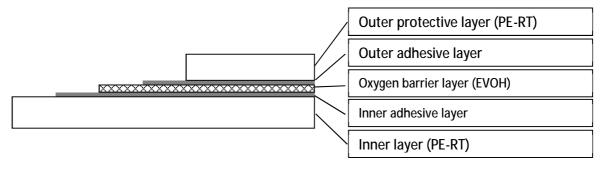
The inner and outer adhesive layers are of the same material as are the inner stress bearing layer and the outer layer.
