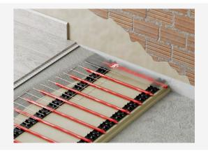
The panels must be installed side by side using the side rails to connect them.
