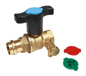
Ball valve, with female threaded-press connections (for copper pipe complying with EN 1057; for stainless steel pipe complying with EN 10217-7 and EN 10312; for carbon steel pipe complying with EN 10305-3), with drain cock with hose connection Ø 9 mm, for pipes with high insulation thickness, specific for domestic water. Full port.
