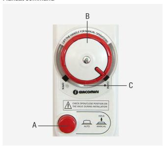
To initiate the actuator manually, keep the red "A" button pressed down and turn the red "B" knob to the desired position.
