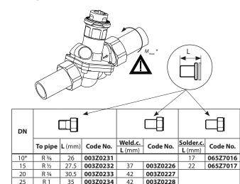
R 1 1/4 \* M<sub>max</sub> for DN 10 is 35 Nm
